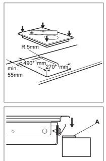
Place the sealing gasket A all around the edge of the cut out.
